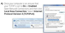
B) If your computer is already on a network, ensure that you have set it to a Static IP Address on the interface. (Example: 192.168.0.88 and the Subnet Mask address as 255.255.255.0.)
